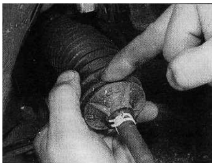
11.2 Checking a steering gear gaiter
