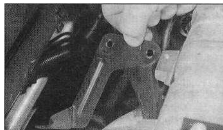
20.2b ... and remove the air cleaner mounting bracket from the top of exhaust manifold
