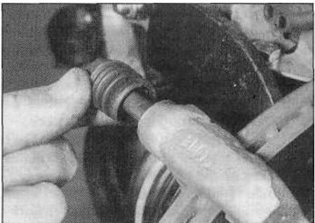
4.9 While the caliper is removed, check the condition of the guide pins and gaiters - Girling caliper shown
