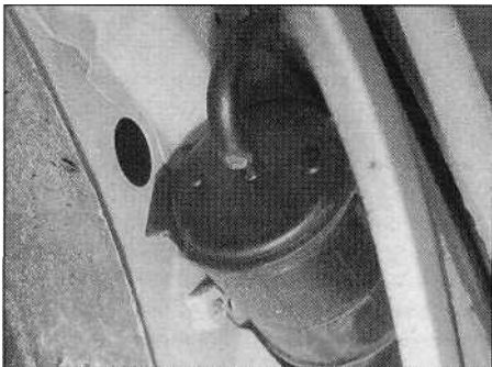
2.5 Peel back the wheel arch liner to gain access to the charcoal canister from underneath the wing
