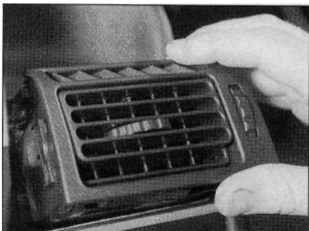
10.1 Withdrawing a facia side vent
