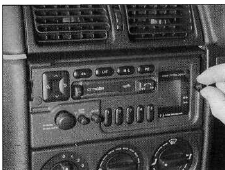
21.2 Remove the rubber plugs ...
