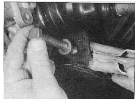
6.5a Slacken and remove the lower suspension arm front pivot bolt...
