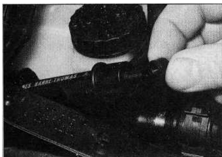
31.4c Removing the heater outlet hose bleed screw (screw located in extension hose)
