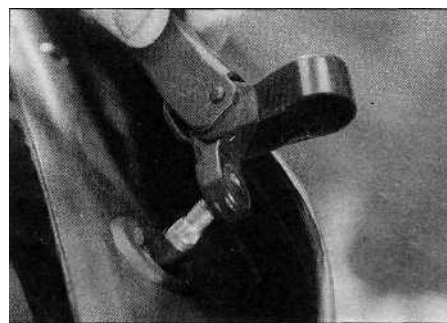
17.2b ... and remove the wiper arm from the spindle
