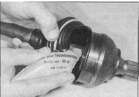
3.21 f Pack the joint with the grease supplied, working it well into the ball tracks while twisting the joint, then locate the gaiter outer lip in its groove on the outer member
