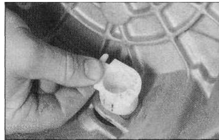
6.7a Clip the lower pivot bush into position in the transmission housing ...
