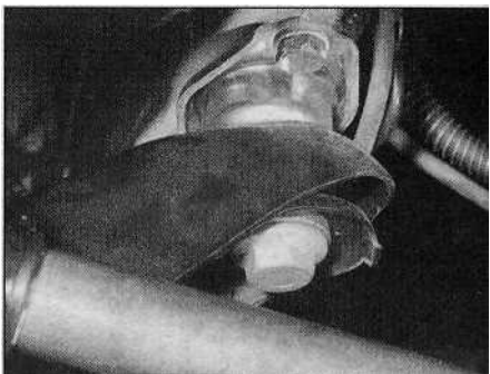
10.9b ... and front mounting bolt
