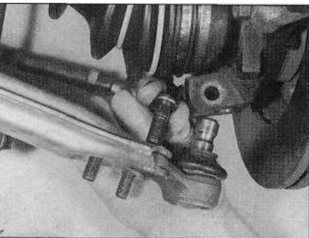
7.2a Remove the three retaining bolts ...
