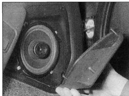
22.2 Remove the grille to gain access to the relevant speaker
