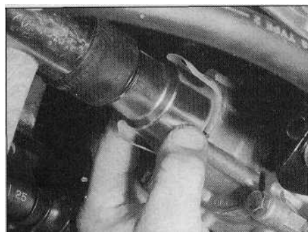
4.8b ... and tap it into position using a tubular drift
