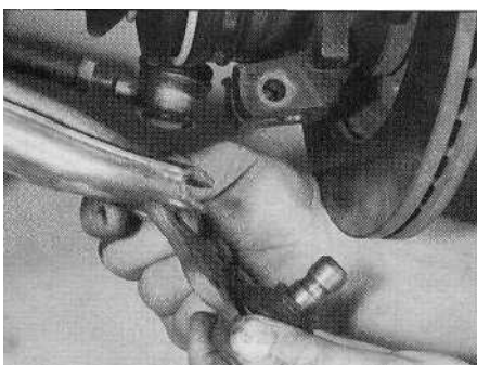
7.2b ... and remove the lower arm balljoint
