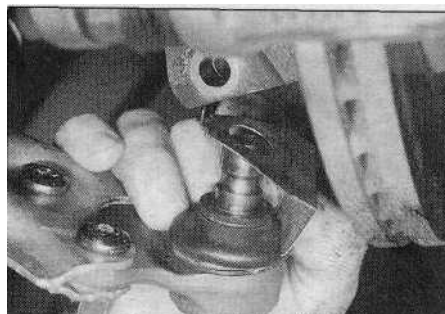
6.4 Release the balljoint from the swivel hub, and remove the protector plate from the balljoint shank
