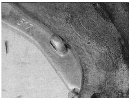
9.12 Check that the handbrake lever stop-peg is correctly positioned against the shoe edge
