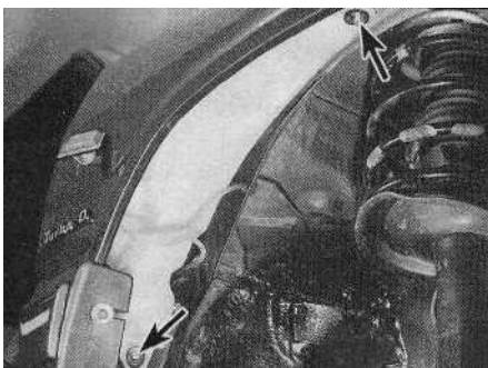
20.6a Undo the two retaining bolts (arrowed)...
