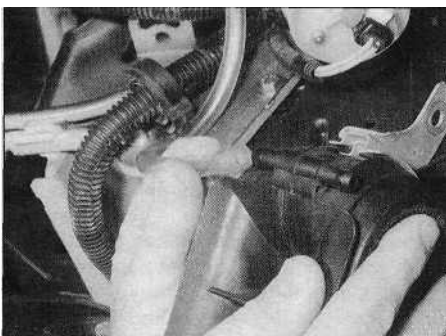
15.3b ... then remove the horn, disconnecting it from its supply pipe
