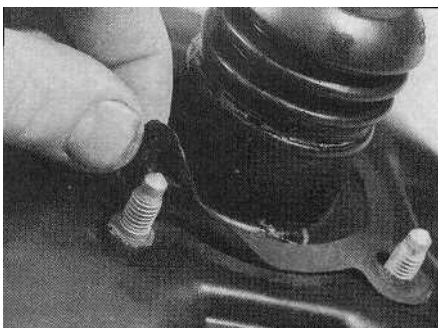
15.11 Prior to refitting, fit a new sealing gasket to the rear of the servo unit
