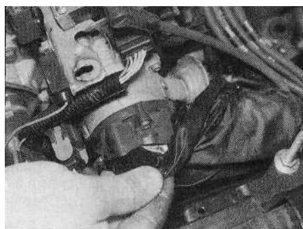
8.2a Peel back the waterproof cover ...
