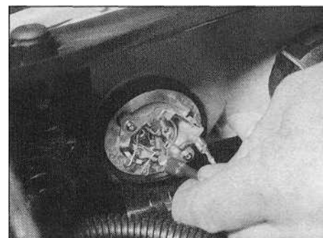
5.3a Disconnect the wiring connectors from the headlight bulb ...
