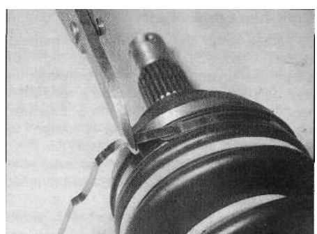
3.21 h Bend the clip end back over the buckle, then cut off the excess clip
