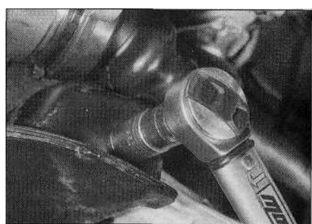
6.12 With the vehicle resting on its wheels, tighten the lower arm front pivot bolt to the specified torque setting
