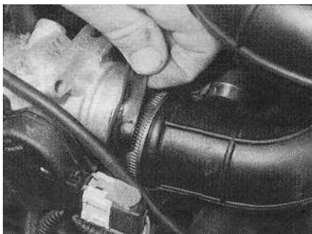
12.7b ... then disconnect the duct and recover the rubber sealing ring
