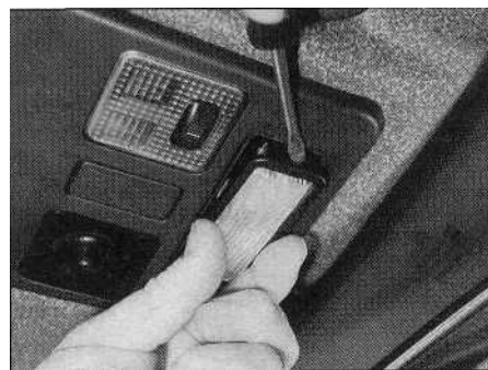
6.2a Prise the courtesy light out of position ...
