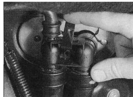
2.34 Remove the metal clip from the top of the heater matrix connector on the engine compartment bulkhead ...
