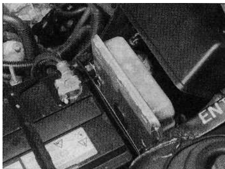
17.16 Unclip the lid from the plastic box to gain access to the ECU
