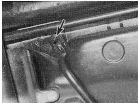
6.9b Fuel tank support rod retaining nut...
