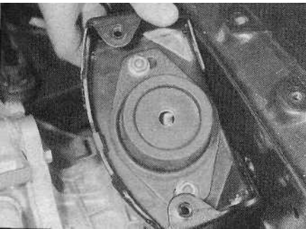
7.18b ... then undo the two retaining bolts and remove the mounting bracket assembly
