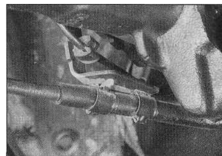
19.5 Handbrake cable trailing arm bracket
