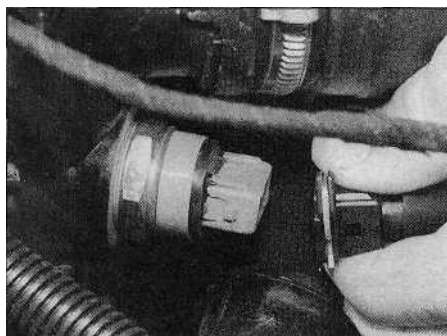
3.4 Disconnecting the cooling fan switch wiring plug
