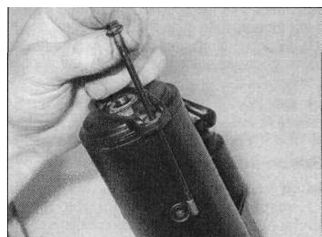
17.4a Remove the through-bolts ...
