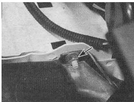
2.4a Undo the intake duct front retaining nut (arrowed)...
