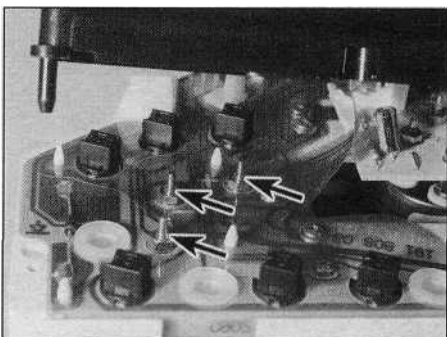
10.11 Temperature gauge retaining nuts (arrowed)
