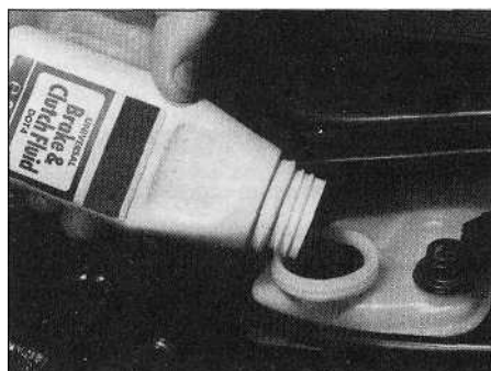
3.12 Topping-up the brake fluid level
