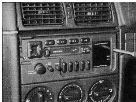
21.3a ... and undo the two radio/cassette unit retaining screws
