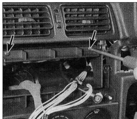
9.3a Undo the two retaining screws (arrowed)...
