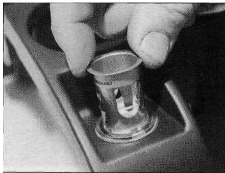
13.4a Release the retaining tangs, then withdraw the metal insert...
