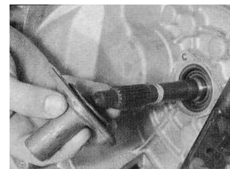
4.25b ... refit the guide sleeve over the input shaft...
