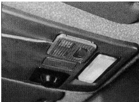
6.6a Carefully prise the map reading light out of the overhead console ...
