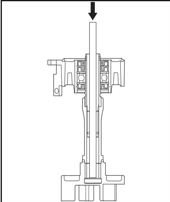
**Driven coupling shaft removal**
