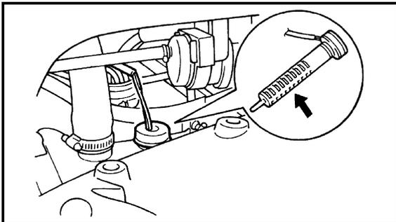
**OIL INJECTION SYSTEM****Oil filter inspection**
