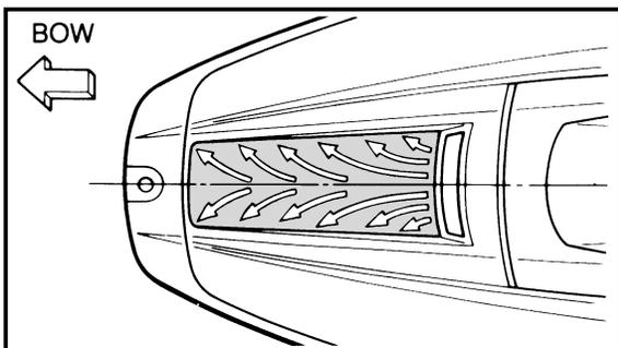
2. To prevent water from entering the urethane foam, apply silicone sealant to the inside of the hole as shown.
