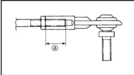
**Steering cable (jet pump side) installation**
