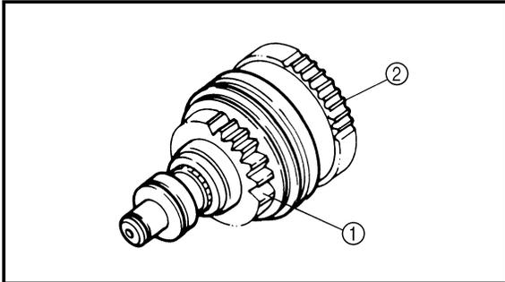
**Starter clutch assembly inspection**
