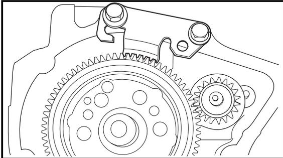
**Flywheel magneto removal and installation**
