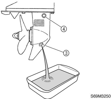
5. Check the oil for metal, discoloration, and viscosity. Check the internal parts of the lower case if necessary.
