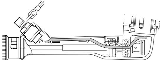
3. Install the tiller handle assembly to the upper case, and then tighten the bolt ③ to the specified torque.
