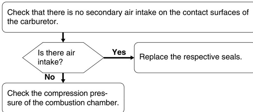
**Symptom: The engine idle speed is not steady, but increases or decreases.**
