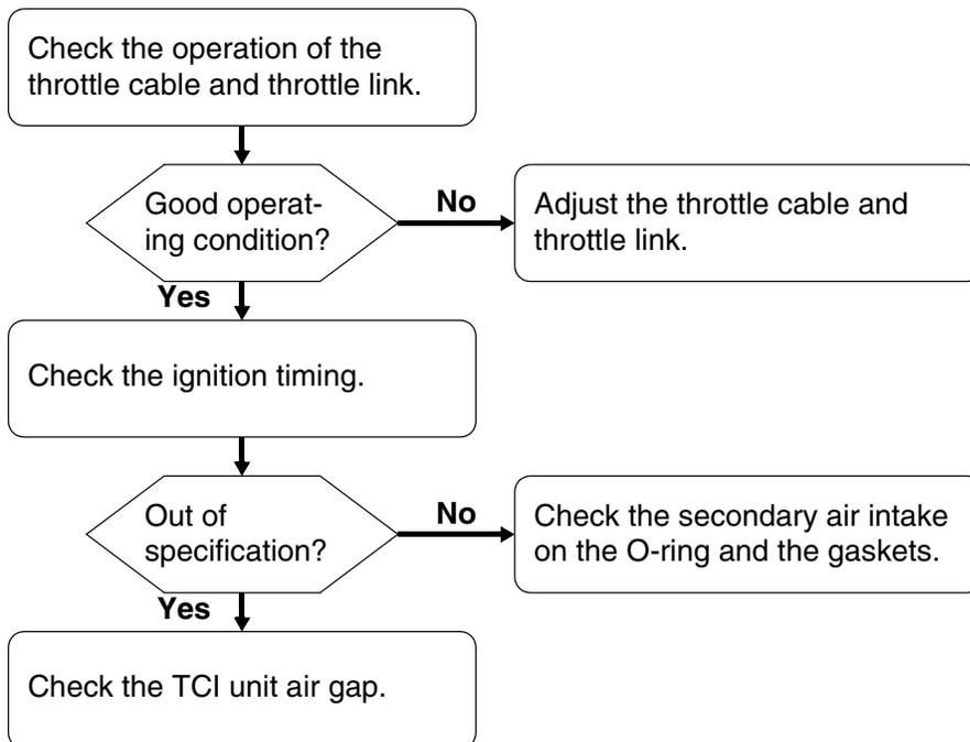
**Symptom: Engine does not accelerate when the throttle is opened quickly.**
