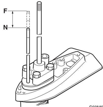
2. Install the lower unit to the upper case.
