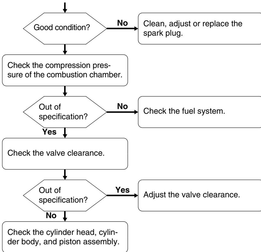
**Symptom: Engine can be started, but does not remain on.**
