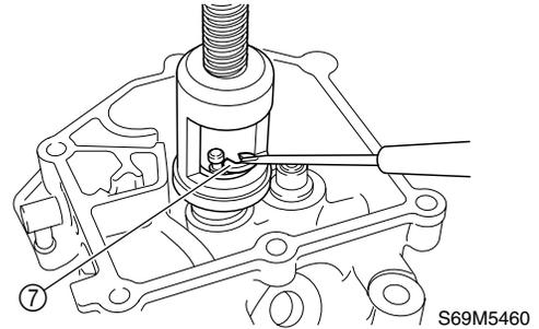
4. Lightly tap the valve spring retainer with a plastic hammer to set the valve cotter securely.
