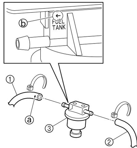
**TIP:** Connect fuel tank breather hose 1 (1), which is identified by the mark (a), to the water separator outlet with the arrow mark (b).
