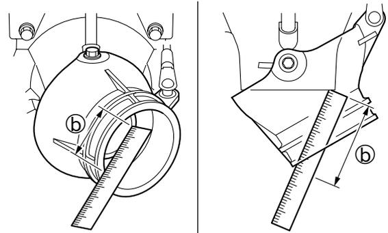
7. If the jet thrust nozzle steering angle cannot be properly adjusted using the cable joint at the steering master end, adjust the cable joint at the jet pump end so that the difference of distances ① and ② is within specification. See "Steering cable installation (jet pump end)" (8-17).
