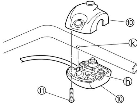
Left handlebar switch screw (11):
