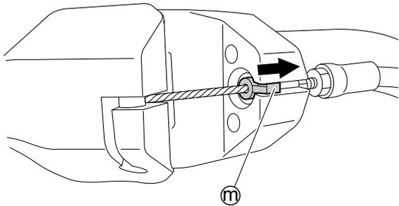
12. Install the corrugated tube (14) onto the throttle cable (3), and then route the throttle cable (3) and left handlebar switch lead (1).
