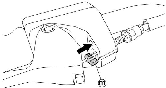
8. Pull the throttle cable (3) in the direction of the arrow shown.
