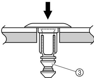
4. When reinstalling a rivet, hold the rivet flange (a) with both hands and push the rivet pin perpendicularly against a hard flat surface until the pin protrudes from the top of the rivet.
