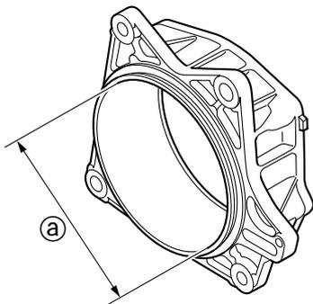
Impeller housing inside diameter @:
