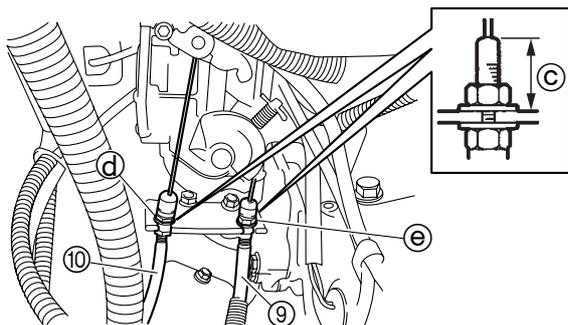
Choke cable and throttle cable guide installation position (C):
