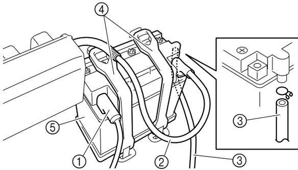
3. Check the battery electrolyte level. If the level is at or below the minimum level mark ①, add distilled water until the level is between the maximum level mark ② and minimum level mark ①.
