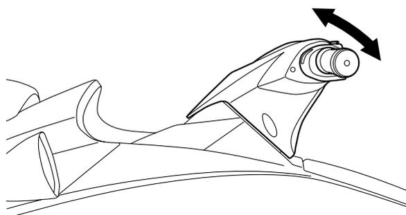
2. Check for excessive play of the handlebar. Check the bushings, bolts, and nuts if there is excessive play. See "Handlebar and handlebar switch assy." (8-2).
