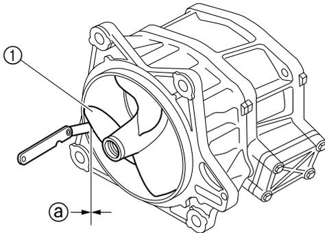
Impeller-to-housing clearance ②:
