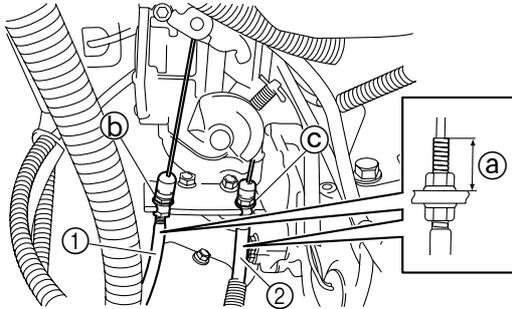
Choke cable and throttle cable guide installation position ①:
