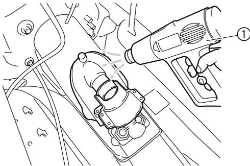
2. Once the adhesive has softened, use a flat head screwdriver to remove the joint ② from the hull.
