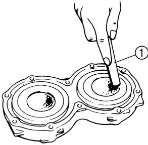
2. Check the cylinder head water jacket. Clean or replace the cylinder head if there is corrosion or mineral deposits.
