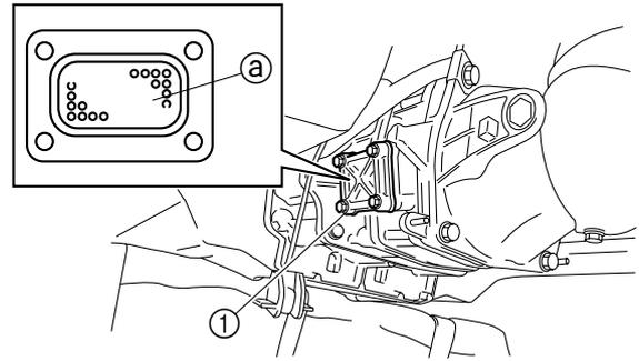
3. Install the water inlet strainer mesh ② and water inlet strainer cover ①. See "Jet thrust nozzle, impeller duct, and impeller housing" (6-5).
