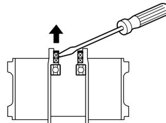
**TIP:** Remove the oil seals using a flat head screwdriver.
