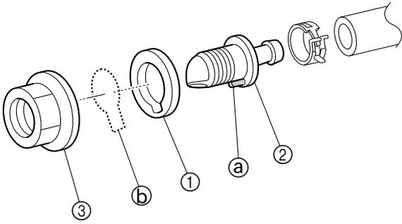
Cooling water pilot outlet nut ③:
