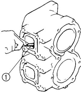
2. Check the cylinder water jacket. Clean or replace the cylinder if there is corrosion or mineral deposits.
