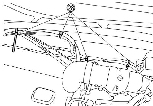
26. Connect the multifunction meter couplers ②⑨, and then install the plastic ties ③⑩.
