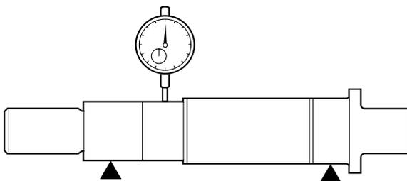
Drive shaft runout limit:
