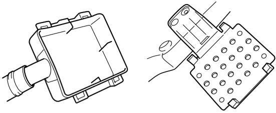
**TIP:** Remove the bilge strainer case ① by pushing the hooks on the bilge strainer inward.
