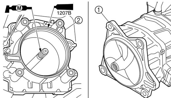
3. Install the jet pump unit ①, and then tighten the bolts ③, ④, and ⑤ to the specified torques.
