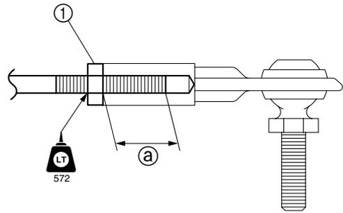
Steering cable set length ② (jet pump end): 14.5 ± 1 mm (0.57 ± 0.04 in)
