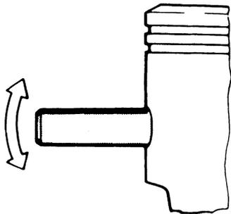
4. Check the piston-pin-to-small-end-bearing-to-connecting-rod free play at the small end of the connecting rod as shown. Replace the piston pin, crankshaft assy., small end bearing, or all parts if there is free play or wear at the small end.
