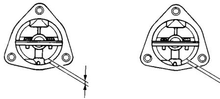
2. Turn out the idle adjusting screw ① until its tips are no longer touching the throttle cable pulley ②.
