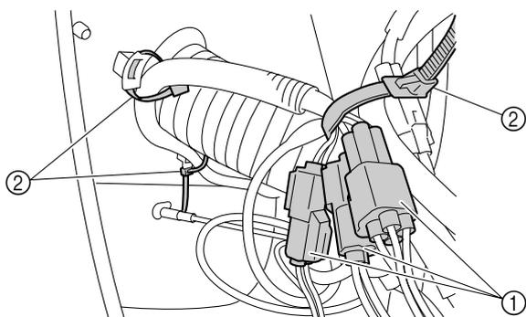
4. Remove the wiring harness from the plastic ties ③.
