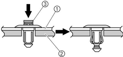
3. When removing a rivet, push the rivet pin ③ in until it clicks and is below the top of the rivet.
