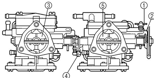
**Choke valve synchronization check and adjustment**
