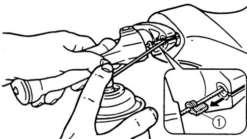
Recommended lubricant: Rust inhibitor
