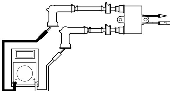
Secondary coil resistance at 20 °C (68 °F)
