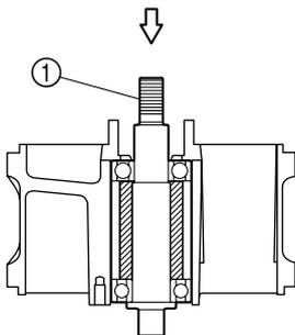
**TIP:** Remove the drive shaft using a press.
