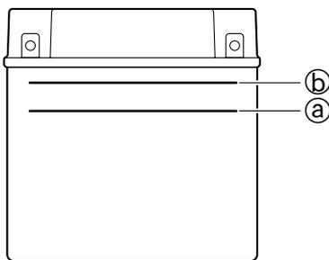
4. Check the specific gravity of the electrolyte. Charge the battery if below specification.
