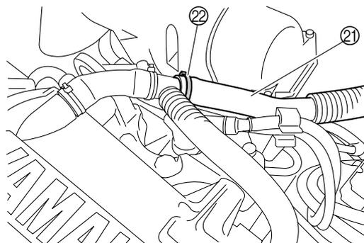
22. Connect the cooling water hose (23), and then install the band (24).
