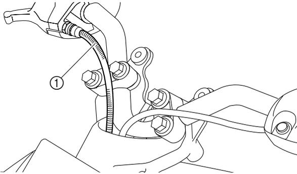
2. Remove the throttle cable ②. **NOTICE:** Make sure to remove the throttle cable seal ③.
