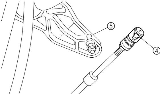
3. Adjust the steering cable. See “Jet thrust nozzle steering angle check” (3-7).
