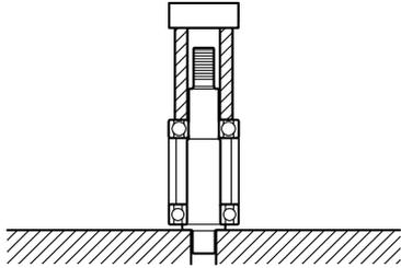
**TIP:** Press the spacer and the front bearing using a pipe of the proper size [more than 60 mm (2.36 in) long and that has an inner diameter more than 24 mm (0.94 in)].
