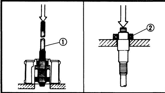
**Drive shaft and bearing removal**
