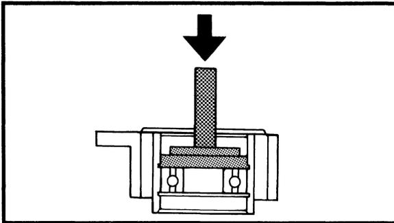
**Bearing removal and installation**
