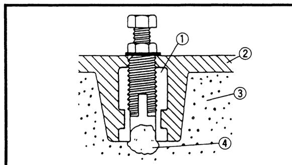
2. Use a 9.4 mm (0.37 in) drill for the final drilling.
