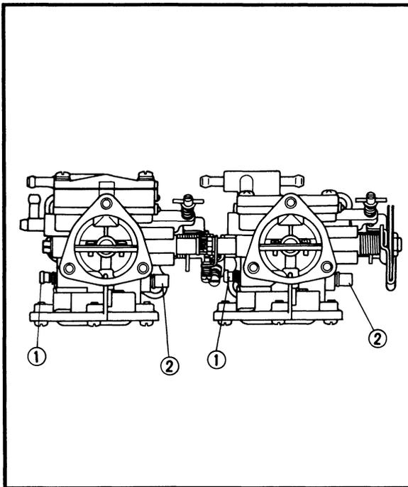
**High and low speed screws adjustment**
