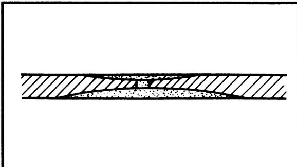
**Hull damage (punctured)**
