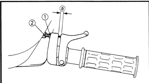
**Throttle cable inspection and adjustment**
