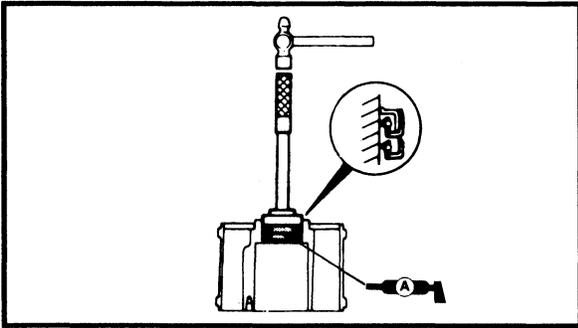
**Oil seal and bearing installation**
