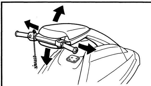
**Steering pole pivot shaft bushing inspection**
