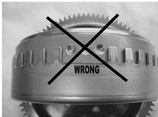
Be sure to align the encoder wheel with the drive pin on the crank gear.
