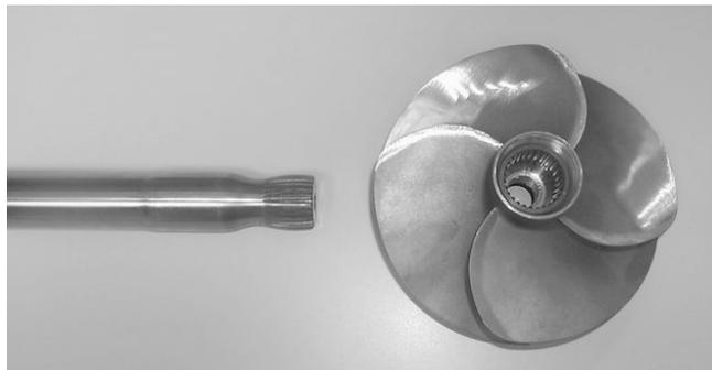
There is also a new four-blade stainless steel impeller that delivers improved acceleration, higher top speed and less cavitation.
