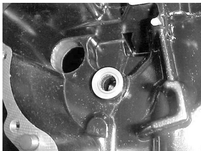
Be sure to install the cam chain tension guide on the crankcase and the cam chain around the crank gear before assembling the crankcases. If not, you will be taking them apart again
