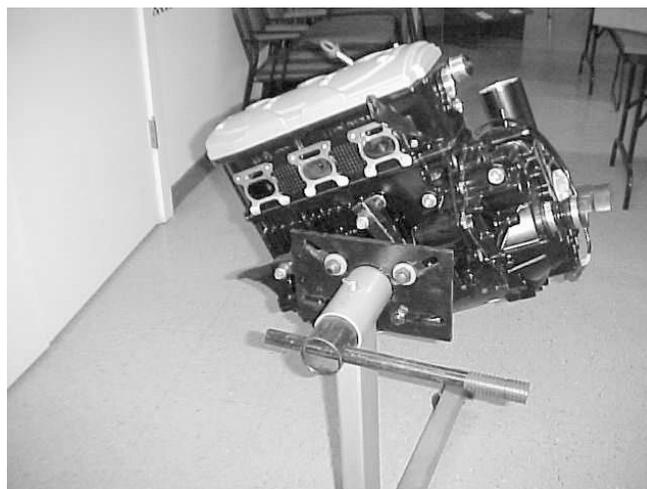
As stated before, if the head does not need to be disassembled for repairs, it can be removed as an assembly. Before removing it, stake the crankshaft and the camshaft, this makes reassembly much easier.
