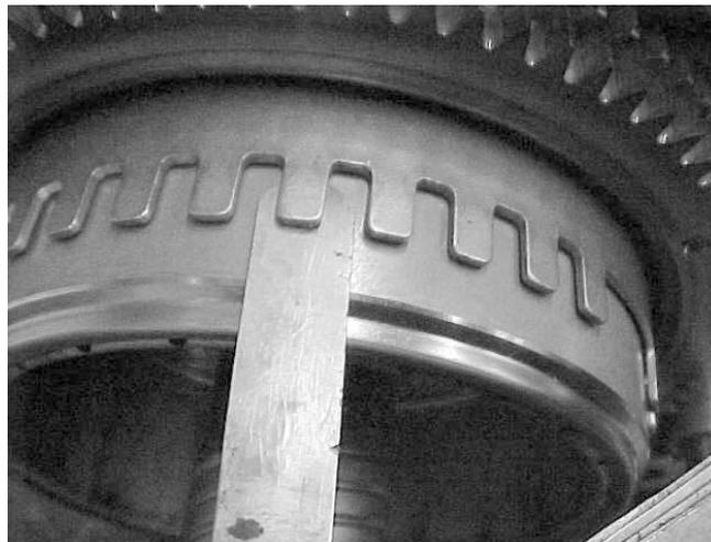
Install the washers correctly on the starter drive.
