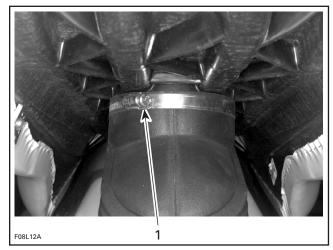
1. Loosen gear clamp
