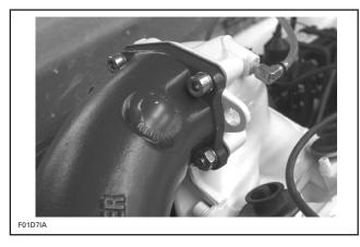
Remove retaining screw no. 20 of tuned pipe head.
