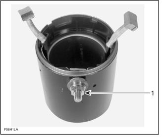
1. Loosen nut and remove washers
