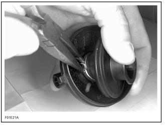
Loosen clamp to separate valve from bellows.
