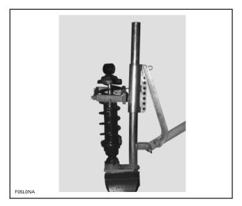
Compress spring and remove cup no. 13.
