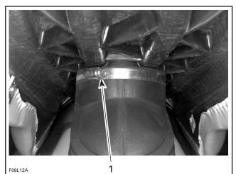
1. Loosen gear clamp
