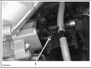
**947 ENGINE** 1. Idle speed screw
