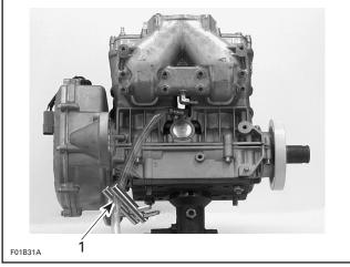
717 ENGINE 1. Oil return hose blocked with hose pincher
