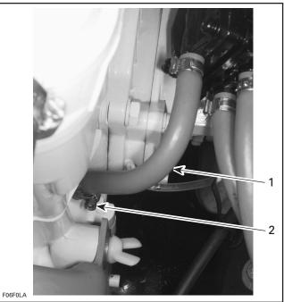
TYPICAL 1. Pulse line 2. Loosen gear clamp
