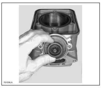
Install the supporting ring **no. 28** with the bevel side facing the O-ring **no. 27**.
