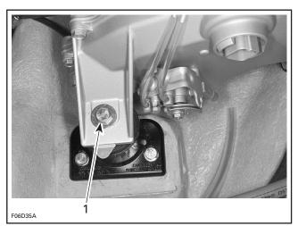
FRONT ENGINE SUPPORT — 787 AND 947 ENGINES 1. Torque to 25 N•m (18 lbf•ft)
