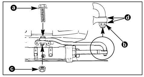
Steering Link Rod Fasteners
