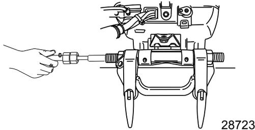
3. Tighten the steering cable nut to the specified torque.
