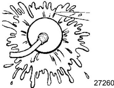
5. Check for a steady stream of water flowing out of the water pump indicator hole. Continue flushing the outboard for 3 to 5 minutes, carefully monitoring water supply at all times.
