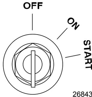
2. **Tiller handle models** - Reduce engine speed and shift outboard to neutral position. Push in the engine stop button or turn ignition key to "OFF" position.
