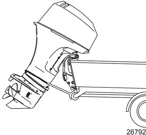
**IMPORTANT:** Do not rely on the power tilt system or tilt support lever to maintain proper ground clearance for trailering. The outboard tilt support lever is not intended to support the outboard for trailering.
