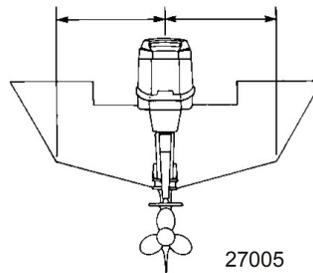
2. Tighten the transom bracket clamp screws.
