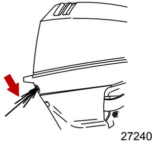
**IMPORTANT:** If no water is coming out of the water pump indicator hole, stop engine and check cooling water intake for obstruction. No obstruction may indicate a water pump failure or blockage in the cooling system. These conditions will cause the engine to overheat. Have the outboard checked by your dealer. Operating the engine while overheated will cause engine damage.
