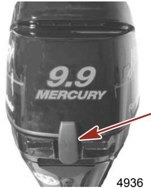
2. Lift front of cowl to clear front latch and push toward the rear to clear rear hook.
