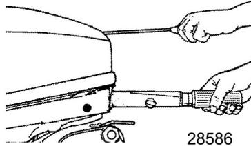
8. **Electric start tiller handle models** - Push the starter button and crank the engine. Release button when the engine starts. Do not operate the starter motor continuously for longer than ten seconds at a time. If the engine fails to start, wait 30 seconds and try again.
