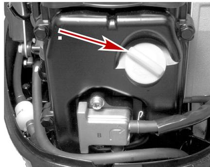
2. Idle engine for five minutes and check for leaks. Stop engine and check oil level on dipstick. Add oil if necessary.
