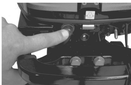
6. **Cold engine** - Pull out the choke knob for starting. Push in the choke knob after engine starts to warm up.
