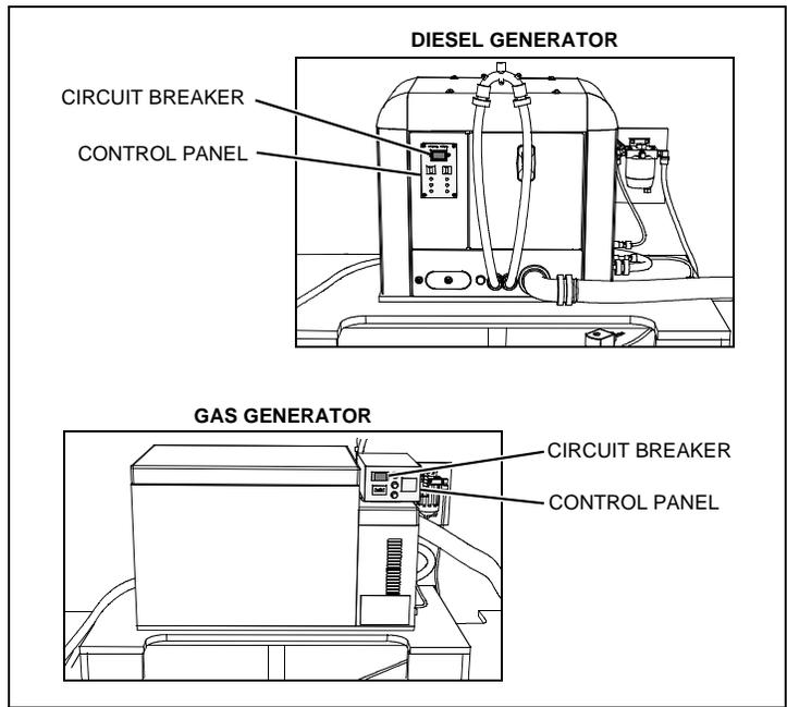
**Generator Remote Start/Stop Panel (If Equipped):** In the galley cabinet above the refrigerator.
