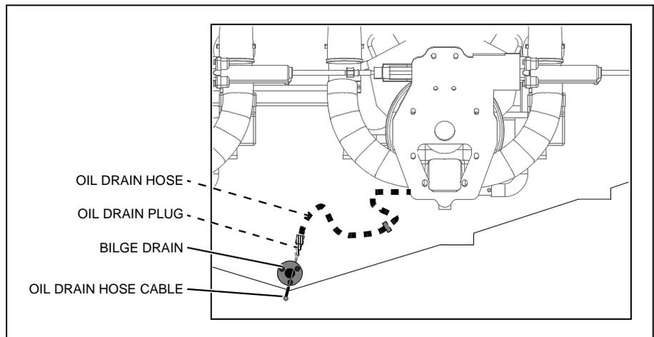
8. Repeat steps 2 through 7 on the port engine's quick oil drain assembly. The only difference being; **the bilge plug assembly, unclipped in step 3, will be used in step 9.**
