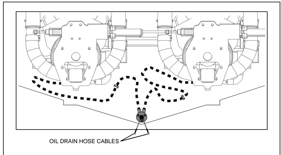
9. Clip the bilge plug swivel clip to both of the oil drain hose cables.
