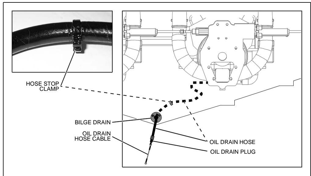
7. Push the oil drain hose and the oil drain plug back into the bilge, but leave the drain hose cable outside of the bilge drain.
