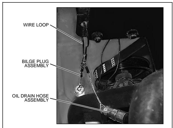
3. Unclip the bilge plug swivel clip from the cable on the end of the oil drain hose.
