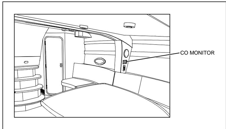
**CO Monitor - Aft Berth:** Located on the port side ceiling of the aft berth.
