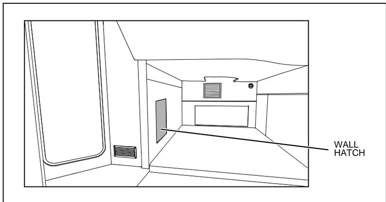
**Engine Hatch Lift Hydraulic Fluid Reservoir (If Equipped):** Located on the engine room wall, forward of the port engine.
